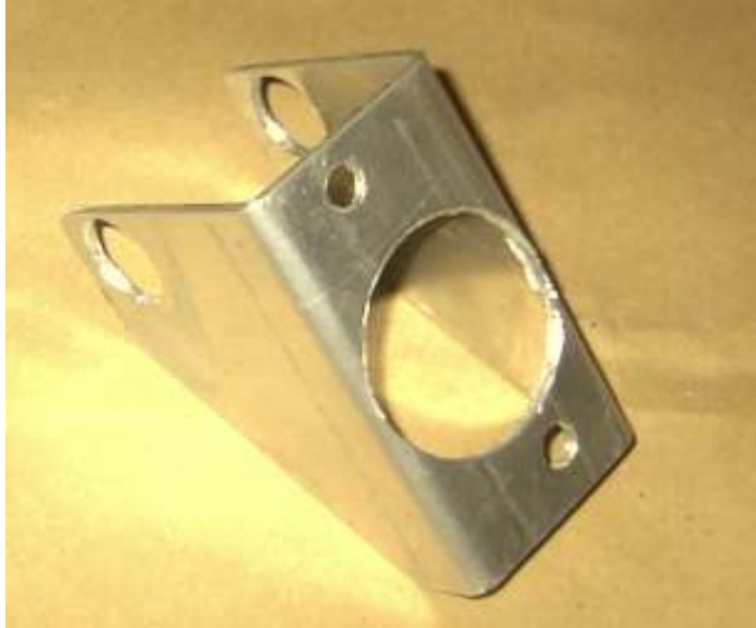
Left Knuckle Bulkhead shown
